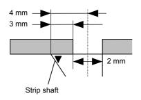
Printing in strip issue mode is stopped at the position where the distance from the middle point of the label-to-label gap to the end of the strip shaft is 4 mm, since the label-to-label gap is assumed to be 2 mm.
