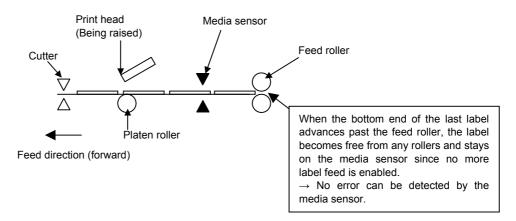
(2) While a cut issue is performed with the print head raised, raising the print head may become disabled due to temperature rise of the solenoid.
