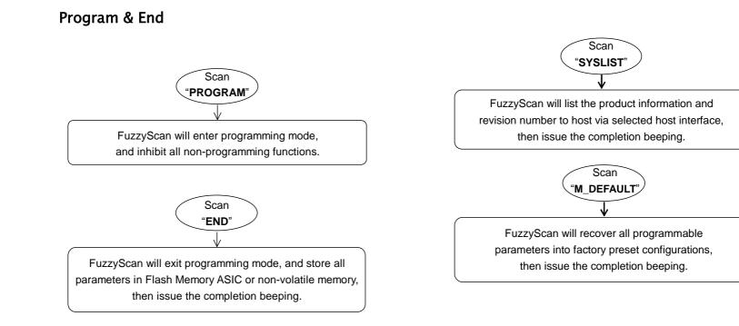
Please note that the FuzzyScan will take 3-4 seconds to store parameters in internal Flash Memory ASIC or non-volatile memory after you scan the "END". Please don't turn off the power before the completion beeping. It may destroy all configured parameters.
