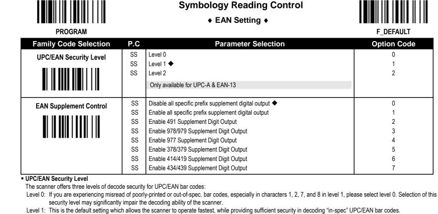
Level 2: If you failed to read poorly-printed or out-of-spec. bar codes in level 1, please select level 2. This is the most aggressive setting and may increase the misread.
