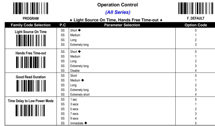
• The Light Source On Time is a pre-defined light source time out counter for Alternative Mode, Presentation Mode and Level Mode. The scanner keeps the light source on till the pre-defined light source on time is up. You can adjust this parameter to meet your own application requirement.
